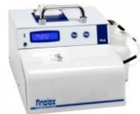
The NutraScan Artificial Gut can be connected to a number of analytical instruments whereby an extract from the digest can be collected and an analysis for specific compounds can be made.
