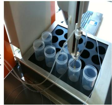
The NutraScan Artificial Gut can be used to automate several of the steps required for measuring TDF. The initial digestion with alpha amylase at 90°C is performed external of the NutraScan. This digest can then be added to the NutraScan reaction cups where the addition of buffers, other enzymes, rinsing and filtration can be performed automatically.
